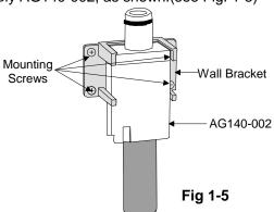
5. Install AG140-002 into 1-1/2" (or 2") drain pipe. (see FIG 1-6)
