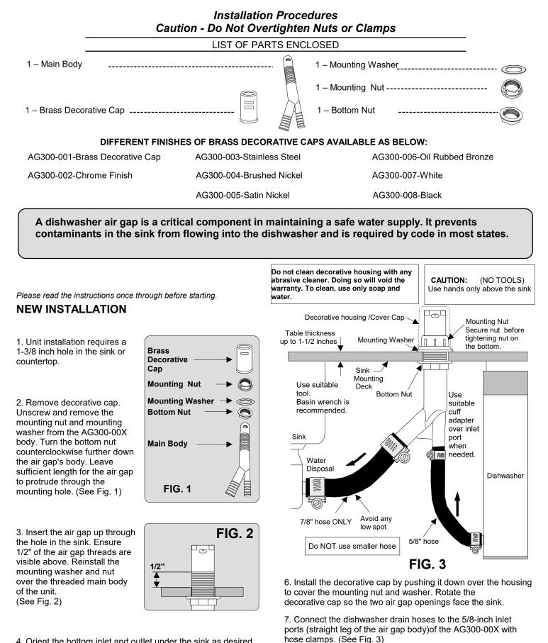
4. Orient the bottom inlet and outlet under the sink as desired. Then, pull down on the air gap while tightening the bottom nut clockwise. DO NOT OVERTIGHTEN.
