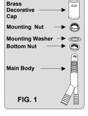
3. Insert the air gap up through the hole in the sink. Ensure 1/2" of the air gap threads are visible above. Reinstall the mounting washer and nut over the threaded main body of the unit. (See Fig. 2)
