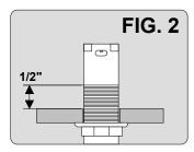
4. Orient the bottom inlet and outlet under the sink as desired. Then, pull down on the air gap while tightening the bottom nut clockwise. DO NOT OVERTIGHTEN.
