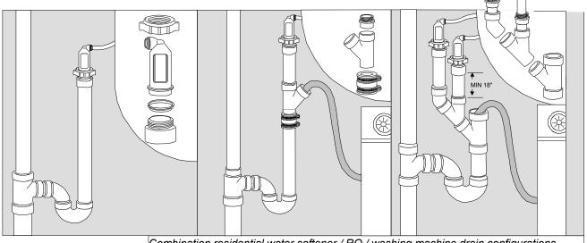
Combination residential water softener / RO / washing machine drain configurations
